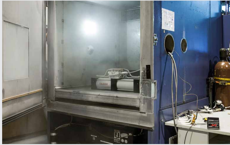
A2A Booster undergoing Low Temperature cycle testing
